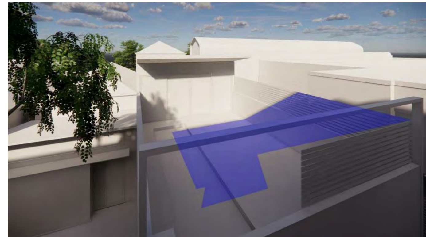
316 ANGAS STREET L1 REAR (NORTH) P.O.S SUNSHADE ANALYSIS: PROPOSED DEVELOPMENT 11AM JUNE 21
